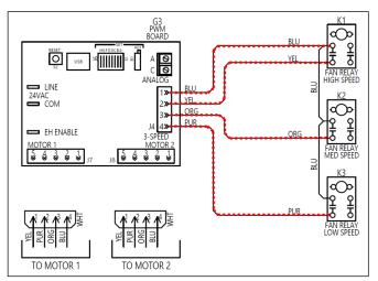
Figure 40 - Remove low voltage signal wires to motor(s)
