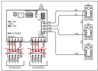
Figure 39 – Remove Motor Signal Wires
