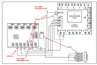
Figure 6 - Sync PWM Electrical Connections
