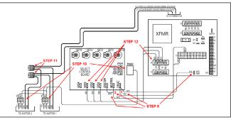
Figure 68 - Select PWM Electrical Connections
