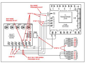
Figure 24 - Select PWM Electrical Connections
