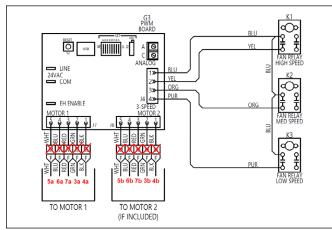
Figure 15 – Remove Motor Signal Wires
