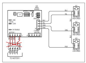
Figure 33 – Remove Motor Signal Wires
