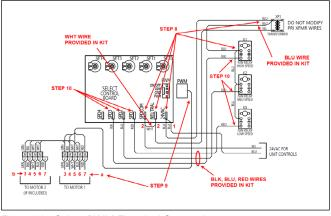
Figure 18 - Select PWM Electrical Connections
