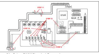
Figure 61 - Select PWM Electrical Connections
