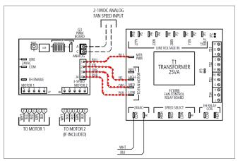
Figure 22 - Remove low voltage signal wires to motor(s)
