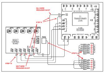
Figure 12 – Select PWM Electrical Connections
