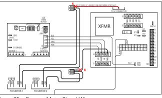
Figure 65 – Remove Motor Signal Wires
