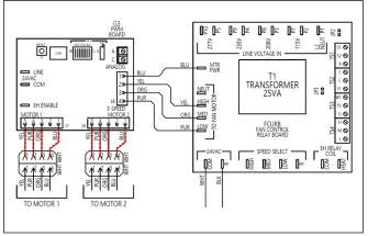
Figure 51 – Remove Motor Signal Wires
