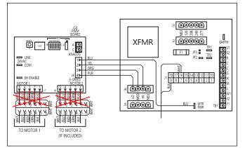
Figure 27 – Remove Motor Signal Wires
