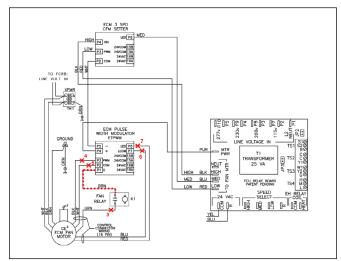
Figure 3 – Remove Motor Signal Wires
