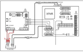
Figure 57 – Remove Motor Signal Wires
