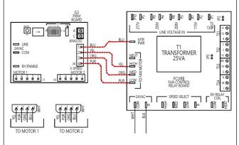
Figure 52 - Remove low voltage signal wires to motor(s)
