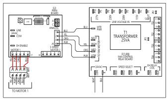
Figure 45 – Remove Motor Signal Wires
