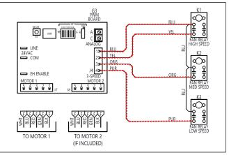
Figure 16 - Remove low voltage signal wires to motor(s)
