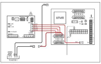
Figure 59 - Remove low voltage signal wires to motor(s)
