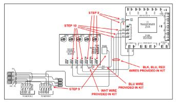
Figure 54 - Select PWM Electrical Connections
