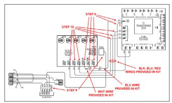
Figure 48 - Select PWM Electrical Connections
