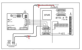
Figure 58 – Remove Motor Signal Wires
