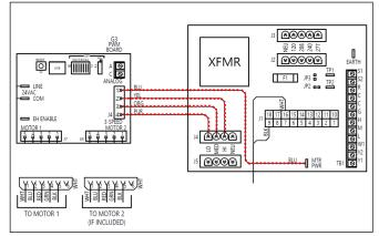
Figure 28 - Remove low voltage signal wires to motor(s)
