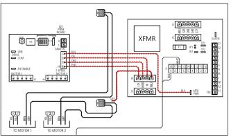
Figure 66 - Remove low voltage signal wires to motor(s)
