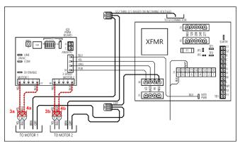
Figure 64 – Remove Motor Signal Wires
