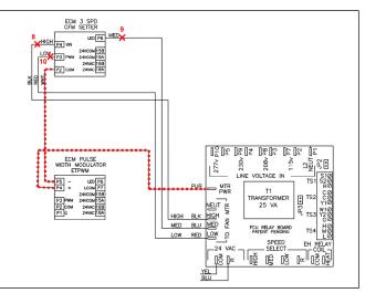
Figure 4 – Remove Fan Control Signal Wires
