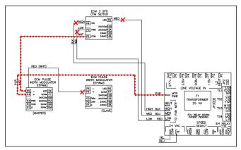
Figure 10 – Remove 2-10VDC motor control signal
