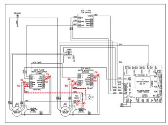
Figure 9 - Remove low voltage signal wires to motor
