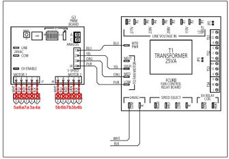
Figure 21 - Remove Motor Signal Wires
